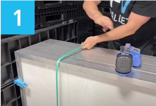
▶ First unitize the load with the vertical bands laid out prior to loading the modules.
