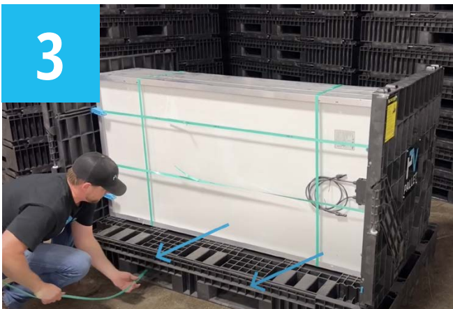
▶ Finally, add two vertical bands—one through each fork pocket. Keep banding to the side of the fork pocket to limit abrasion from forklift tines.
