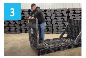
Lift wall until the posts clear the base wall pockets.
