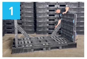
▶ Before loading your Series X, lock the two cross braces firmly in place on one side of the pallet.
