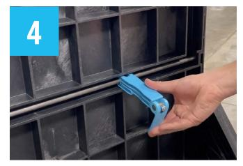
Lock the handle in place by squeezing the front lever back towards the handle.
