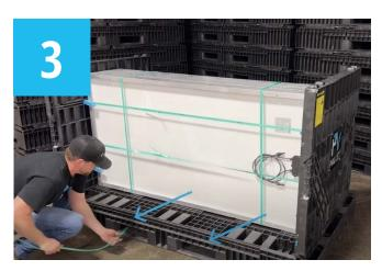
Finally, add two vertical bands—one through each fork pocket. Keep banding to the side of the fork pocket to limit abrasion from forklift tines.
