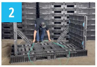
Lay out two bands used for vertical banding that your modules will rest on.
