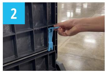
▶ Remove the handle from its stowed position by lifting the front lever, then pulling slightly toward you.
