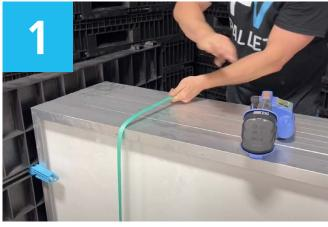
▶ First unitize the load with the vertical bands laid out prior to loading the modules.
