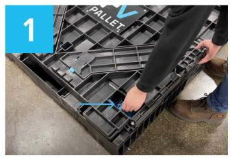
▶ Release the sidewall from the base by compressing either latch and sliding the wall toward you.
